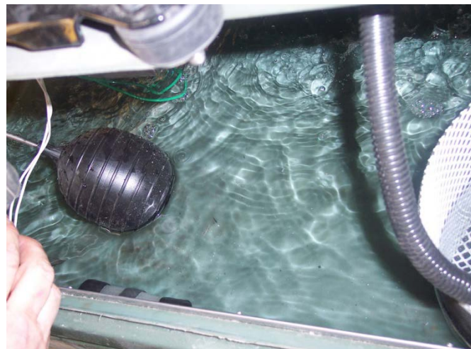
Figure 8: Float to adjust water sump level
