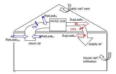
Duct loss and gain components in DOE2.2
